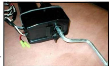
Turn the crank counter-clockwise until the lift has reached its lowest position.
